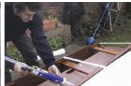
**11** We used clear silicone sealant as a waterproof beading to seal the staples, then draped the covering half over.
