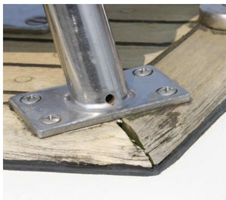
▲ This thin timber decking has lost its caulking compound and the corner is starting to deteriorate
