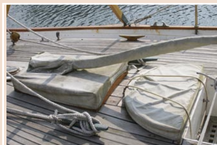
▲ Covers over vulnerable varnish work makes sense but a complete cover will protect more than just the deck
