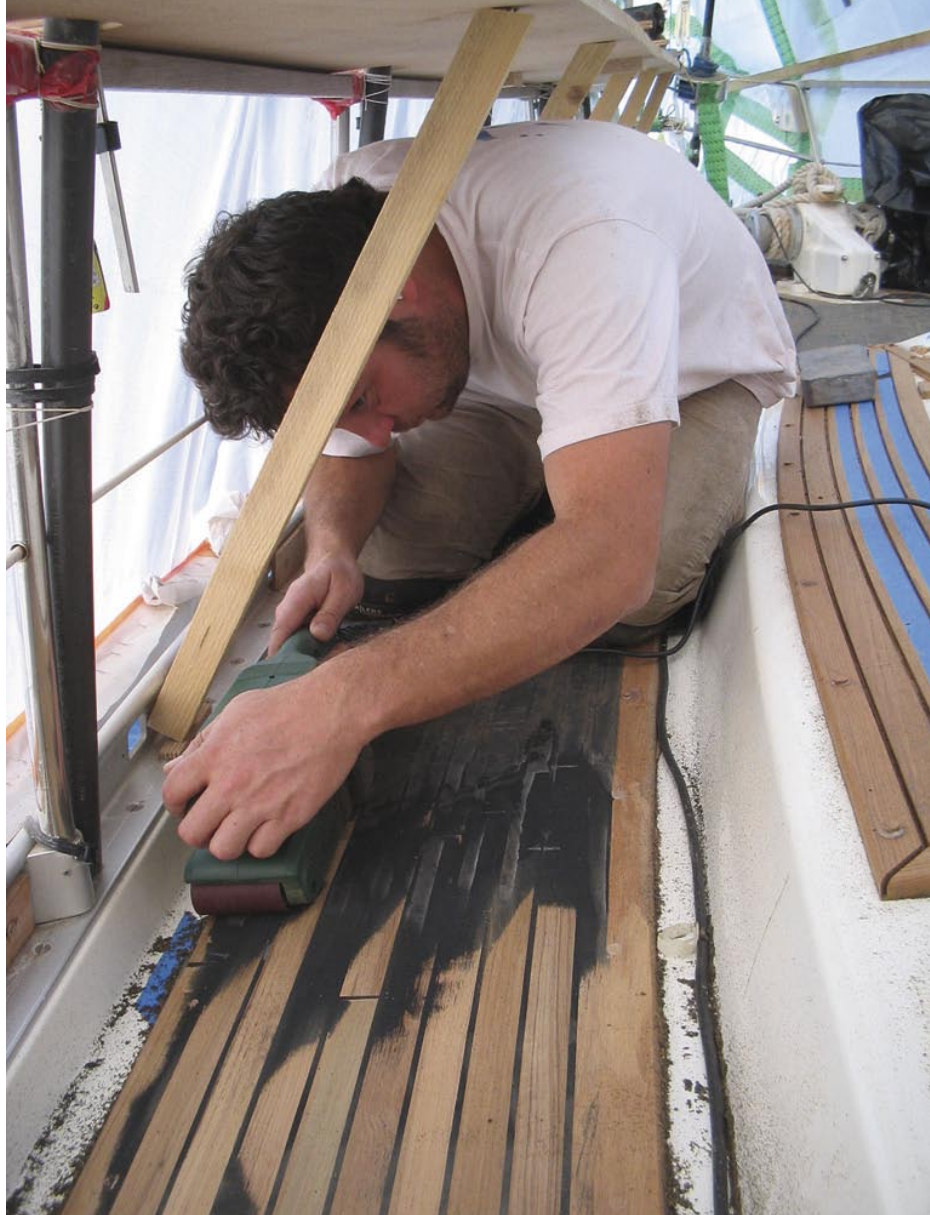
New decks get sanded to get everything finished nice and flush – but it's not a good idea to repeat it too often
