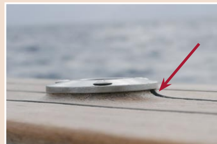
▲ This is what one modern teak deck looks like after only five years of regular cleaning and sanding
