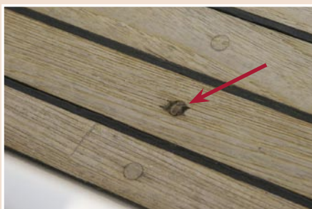
▲ This plug seems to have a problem. It could be loose and holding moisture, or the fastening is corroding
