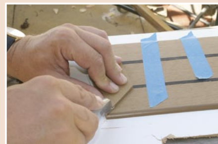
▲ Artificial teak is not the same as the real thing but it is very easy to lay and can just be cut with a knife
