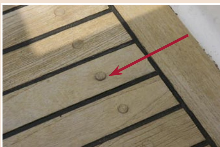
▲ As the decking is very thin, the plugs over the fastenings are even thinner and can lift if the glue fails
