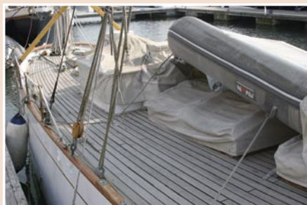
▲ Even more modest pine decks have stood the test of time because they are made of quite thick planking
