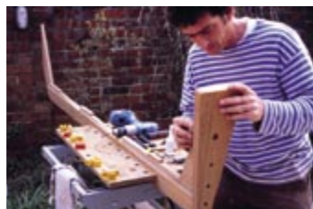
3 The keel, stem and sternpost (note knee) are all glued into one piece, in traditional style, as the boat's backbone
