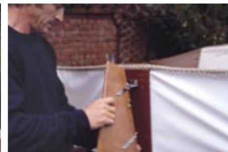
17 Our Oppy gudgeons will get in the way of the outboard and eye bolts will be better. The rudder hangs a little high.
