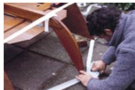
10 Stainless-steel staples (10mm) hold the tensioning tapes in place; these give her her shape before covering.
