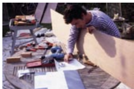
2 Benjy downloaded his plans and began the work of sawing up all the wood into the patterns for assembling the tender.
