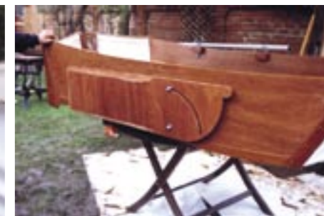
18 The ingenious leeboard is so easy to fit and use and it works, helping Origami to stay on the wind. Voila, she's done!
