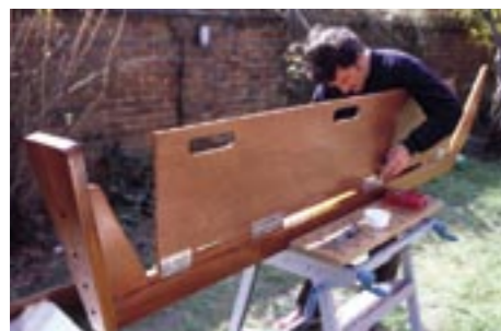
4 The dinghy sole, or bottom boards are of 11mm ply bolted through 4 and 6in (10 and 15cm) stainless hinges, four per side.
