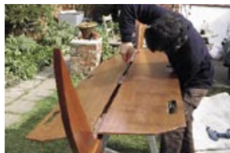
6 The carry holes get rid of some weight and are useful for carrying the dinghy; the boat will be wider than this photo shows.
