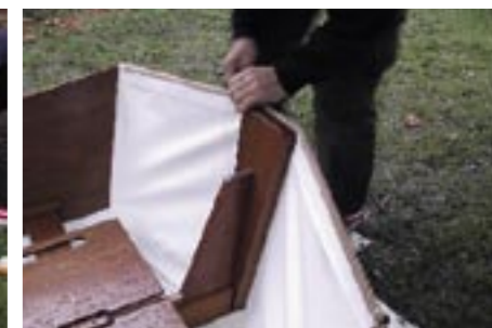
15 With the last transom back screwed in place we sewed on the bolt ropes: buff polyester Posh from English Braids.
