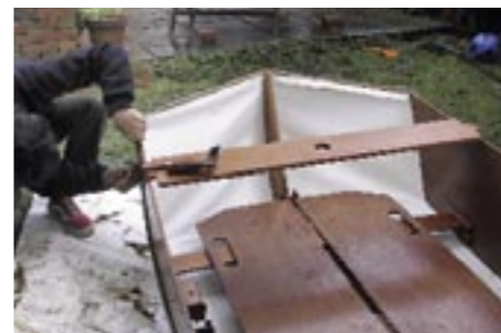
16 The sailing rig requires a tabernacle on the keel and a thwart cut into the bow boards and tensioned back to the keel.
