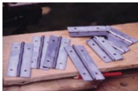
5 These are the hinges cut out from a plain stainless-steel piano hinge from Anglia Stainless, then smoothed off on a belt sander.
