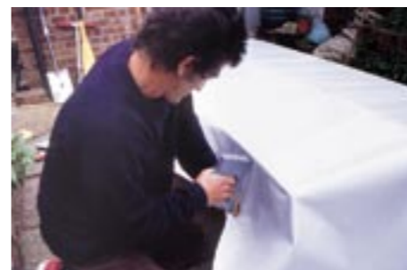
13 We had more than enough PVC polyester canvas to cover the boat. It may come in useful if we ever need a repair.
