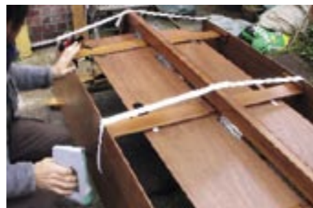
9 Taping up, with strips of PVC polyester. Her boards are held up aft by two swing-out legs to prevent collapse on capsizes.
