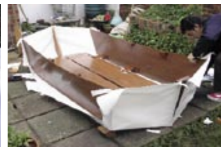
14 With the 'bottom' stapled on we trimmed off the excess with a sharp knife before screwing on the covering pieces
